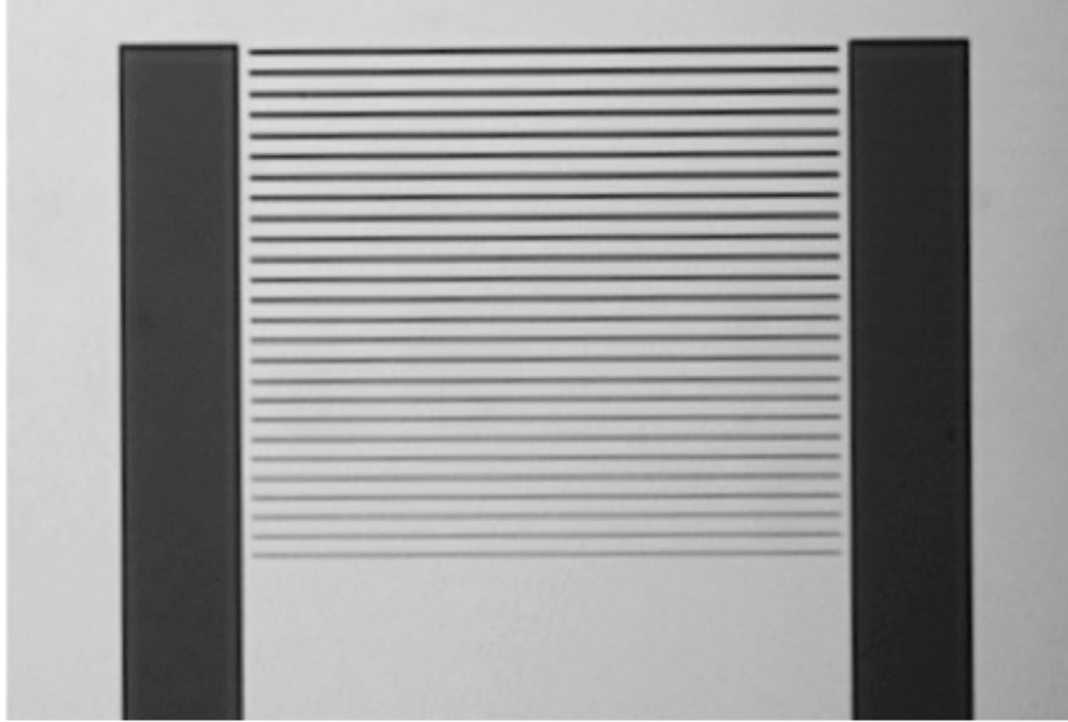
Figure 5.1.3: Scanning electron micrograph image of a fabricated SOS grating coupler.
