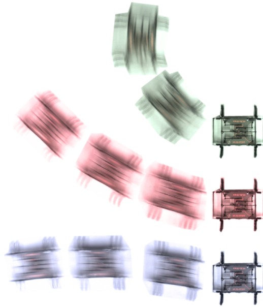
Figure 5.11: The orientation of HAMR-V and HAMR-VP can be controlled by altering the phase of lift DOF input signals, \psi_i . Heading during quasi-static operation is controlled by the left front leg's lift phase \psi_1 , causing right or left turns by tuning phase from \psi_1 = 210^\circ to \psi_1 = 330^\circ , respectively. For dynamic locomotion, two legs are required to affect orientation: \psi_1 for left turns and \psi_2 for right turns (b). In (b) HAMR-V ran at 60Hz gait frequency using \psi_1 = \psi_2 = 270^\circ for nominally straight locomotion (middle), \psi_1 = 210^\circ, \psi_2 = 270^\circ for left turns (bottom), and \psi_1 = 270^\circ, \psi_2 = 330^\circ for right turns (top).
