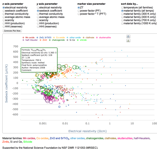
34 35 36 37 38 39 40 41 42 43 44 45 46 47 48 49 50 51 52 53 54 55 56 57 58 59 60 Figure 3: Screenshot of the web-based visualization tool, that permits the simultaneous visualization of four parameters: abscissa, ordinate, marker size and color: Several variables can be chosen as abscissa and ordinate, and measures of thermoelectric performance can be represented by the radius of the data points. To simplify navigation, families of related materials can be displayed or hidden by clicking their legend marker. Further, hovering over a data point intuitively reveals a tooltip with pertinent information: the names and values for the abscissa and ordinate, the chemical composition, the sample form (e.g., polycrystalline, single crystal, nanoparticles), the preparatory route (e.g., ceramic method, arc melting), the author and year, and either the power factor, \kappa zT , or zT value. Clicking on a data point leads the web-browser directly to the source publication via the document object identifier (DOI).
