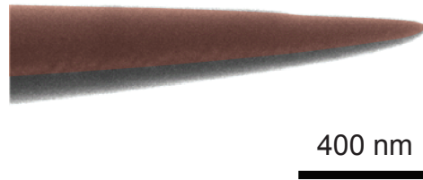
Figure 4.6.1: Scanning electron micrograph of a quartz tip with magnetic coating. The metal coating is overlain in red (false color).
