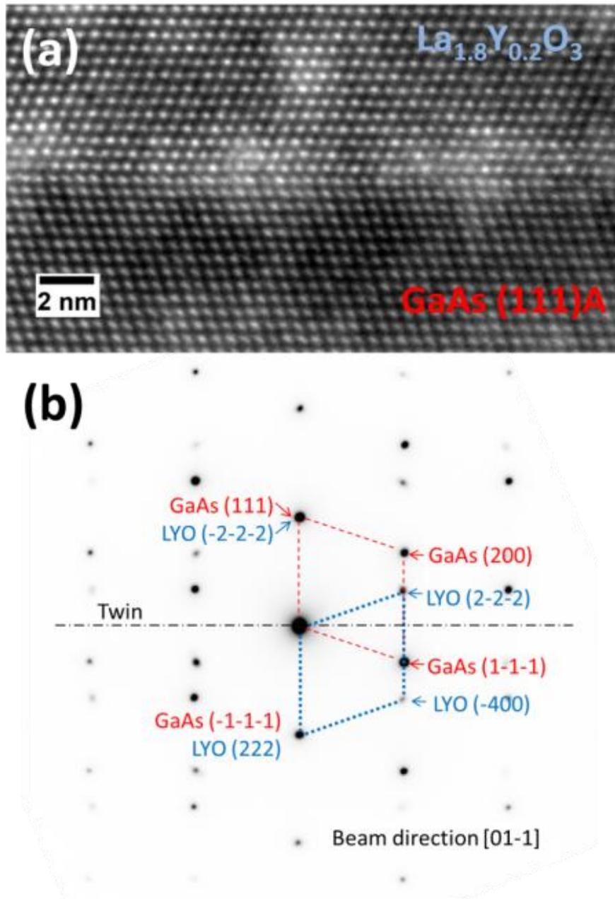
Figure 1. (a) Cross-sectional TEM image of  $\text{La}_{1.8}\text{Y}_{0.2}\text{O}_3/\text{GaAs}(111)\text{A}$  interface, and (b) the corresponding electron diffraction pattern with the electron beam aligned along the  $[01-1]$  direction of GaAs. (“ $\text{La}_{1.8}\text{Y}_{0.2}\text{O}_3$ ” is labeled as “LYO” in the diffraction pattern.)
