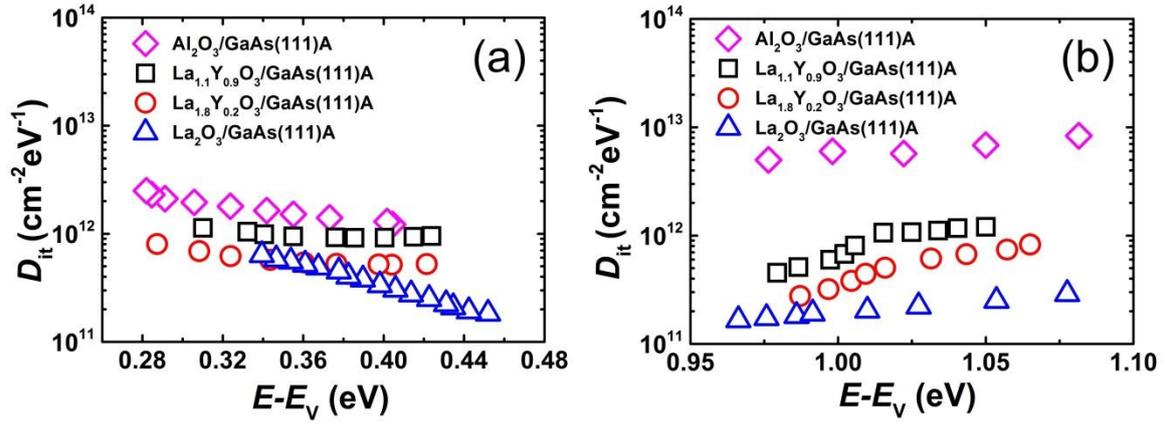
Figure 4.  $D_{it}$  distribution in the GaAs band gap obtained on both (a) p-type and (b) n-type MOS capacitors with  $\text{Al}_2\text{O}_3/\text{GaAs}(111)\text{A}$ ,  $\text{La}_{1.1}\text{Y}_{0.9}\text{O}_3/\text{GaAs}(111)\text{A}$ ,  $\text{La}_{1.8}\text{Y}_{0.2}\text{O}_3/\text{GaAs}(111)\text{A}$  and  $\text{La}_2\text{O}_3/\text{GaAs}(111)\text{A}$  as the interfaces, respectively.
