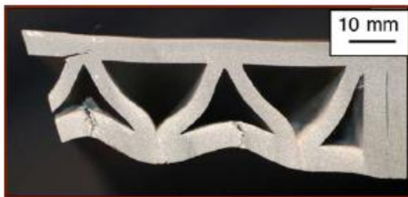
(b) Panel center failure
