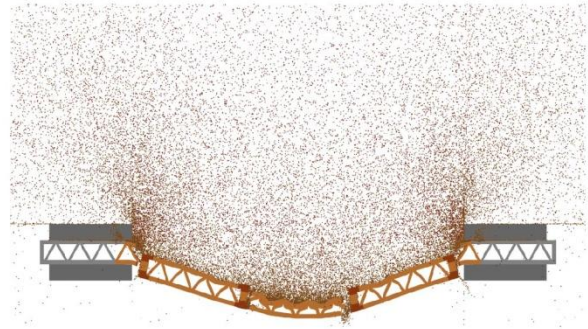
Figure 19. Time resolved interaction of sand particles with a sandwich structure at a stand-off distance of 15 cm. Results are shown for a thin slice of the modeled problem that passes through the center of the test charge and the sandwich structure transverse to the welding direction.
