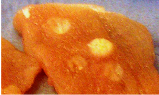
Figure 7.8 Tissue sample ablated with the catheter force sensing RF ablation tool. The lesions are approximately 4 mm in diameter
