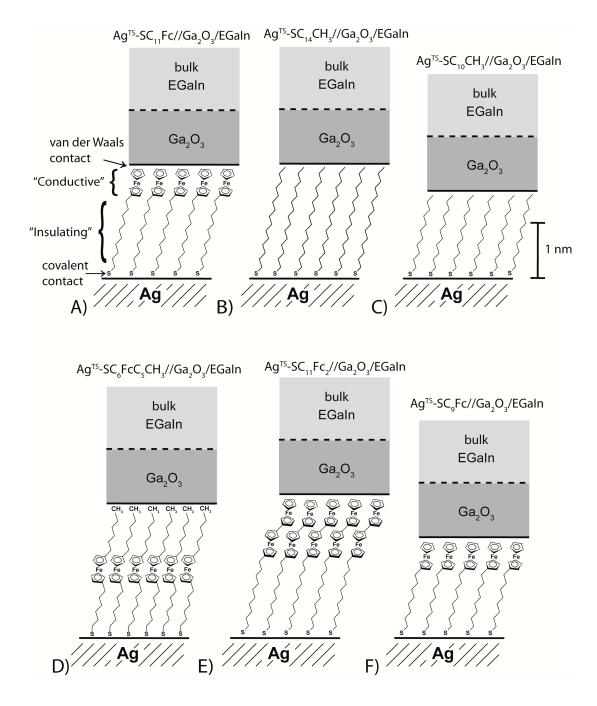
tunneling. Thus, charges encounter a wider tunneling barrier at reverse bias than at forward bias. Since tunneling current decreases exponentially with increasing width of the barrier, a higher current flows at forward bias than at reverse bias, and the junction rectifies.
