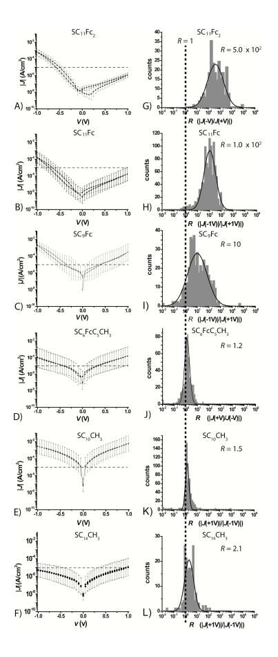
Rectification in Insulators:  $Ag^{TS}$ - $SC_{n-1}CH_3//Ga_2O_3/EGaIn$  (n = 11 or 15). The  $Ag^{TS}$ - $SC_{10}CH_3//Ga_2O_3/EGaIn$  and  $Ag^{TS}$ - $SC_{14}CH_3//Ga_2O_3/EGaIn$  junctions rectify with values of *R* close to unity (Table 3).<sup>23</sup> Although the values of *R* in these junctions are small (*R* = 1.5 and 2.1), a Student's t-test indicated that they differ significantly from unity, and a two-sample t-test indicated that they also differ from one another.<sup>23</sup>
