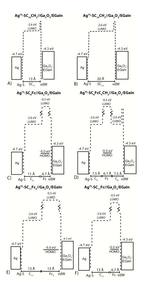
resistance of the layer of  $Ga_2O_3$  is at least four orders of magnitude less than the resistance of a SAM of  $SC_{10}CH_3$  (see Supplemental Information).<sup>23,32</sup> Furthermore, the high dielectric constant of  $Ga_2O_3$  (~ 10)<sup>70</sup> compared to that of SAMs of alkanethiols (2.7)<sup>71</sup> implies that the potential tends to drop along the SAM, rather than the  $Ga_2O_3$ .
