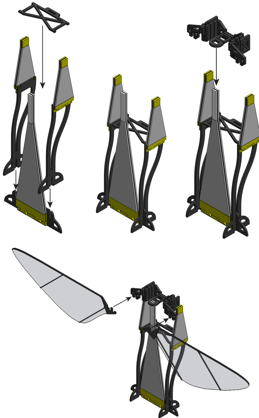
Figure A.7: Assembly process. The side walls of the airframe are inserted into slots in the base piece, then the crossbrace is attached (top left). This results in the completed actuator-airframe structure (top center). The transmission is then mounted to the actuators (top right). Finally, the wings are attached to the transmission (bottom).
