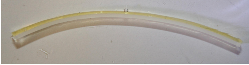
Figure 2.5: PEG-based hydrogel grafted to PDMS acting as an actuator. The width:length ratio is approximately 0.2 and the PEG:PDMS thickness ratio is about 0.3. Complete submersion in deionized water yields a radius of curvature of about 4 cm.
