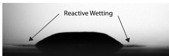
Figure 6.8: (a) Liquid galinstan that has been in contact with a Tin foil surface ( 20\ \mu\text{m} thick) for over 4 days. Reactive wetting can be inferred not only by the slow spreading of the liquid on the surface, but also the signature of the surface material changes occurring around the perimeter of the droplet.
