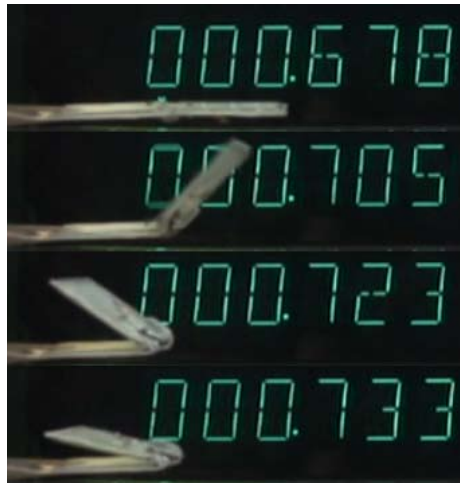
Figure 5.5: Folding sequence of the origami module powered with the eGaIn circuit. The integrated soft curvature sensor measures the angular deflection by detecting the change in resistance, given in Ohms.
