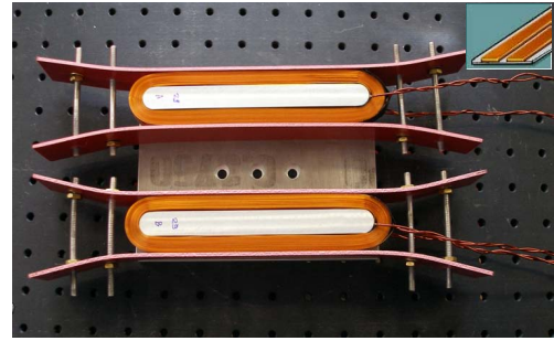
FIG. 1: (Color online) Photography of macroscopic symmetric magnetic guide structure, the inset picture shows the double tape conductor.
