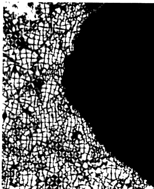
Fig. 9. — Photomicrograph between crossed polars of an aligned DPPC liquid crystal containing 7% water by weight at 96 °C. The sample thickness is 125 μm. The lighter, more birefringent arrays have a period twice that of the dark arrays. Focus is mid-height.
