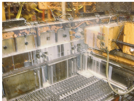
Figure 1. In a process similar to that used by the patient, metalworking fluid (milky appearance) is flowed over auto parts to reduce friction and cool metal tools. As fluids are sprayed over metal parts, a visible aerosol is formed that can be breathed by operators of the machinery unless specific control measures are instituted. Fluids are recycled from large holding tanks. The presence of carbon and water in fluids permits growth of microorganisms, including mycobacteria.
