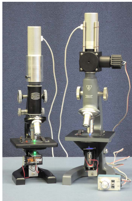
Fig. 1. (Color online) The Spencer (left) and the Bausch and Lomb (right) microscopes. The Spencer microscope is fitted with an iSight camera using a simple aluminum coupler. The eyepiece lens tube of the Bausch and Lomb microscope has been cut to compensate for the additional height of the fluorescence attachment.
