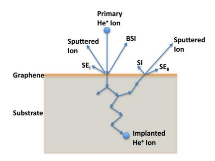
**Figure 2.** Schematic of the interactions of primary energetic He ions with a graphene layer on  $SiO_2$  substrate, showing the production of secondary electrons ( $SE_I$  at the primary beam and  $SE_{II}$  at the secondary scattered ion exiting the surface), back scattered ions (BSI) and secondary ions (SI).
