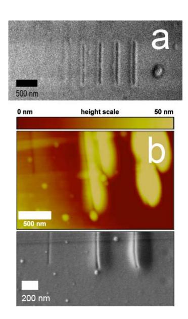
**Figure 6.** a) Helium ion micrographs of a dose variation test pattern in single-layer graphene, on SiO<sub>2</sub> substrate covering a range of linear doses from 3 nC/cm to 15 nC/cm in 3 nC/cm steps (left to right). b) AFM image with corresponding SEM image of a pattern etched with 20, 100 and 200 nC/cm line dose variation (from left to right).
