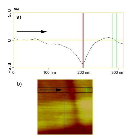
**Figure 7.** a) AFM step profile analysis for the single-layer graphene cut in Fig. 6(b) with a dose rate of 20 nC/cm resulting in a depth of 4 nm. b) AFM image used for the step profile. The profile was taken along the upper part of the image, in the position and direction indicated by the arrow.
