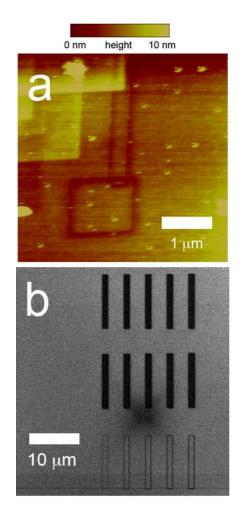
**Figure 4.** a) Test patterns written into a 285 nm SiO<sub>2</sub> film on silicon substrate as measured with AFM and b) Secondary electron image showing etching of boxes and line box patterns.
