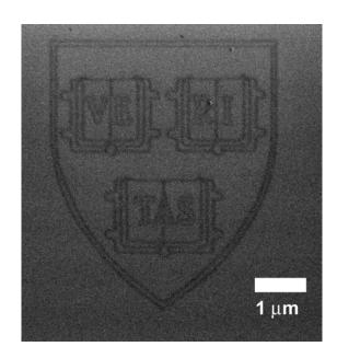
**Figure 8.** Helium ion micrograph of a high resolution Harvard University logo etched by HIL into multi-layer graphene flake.
