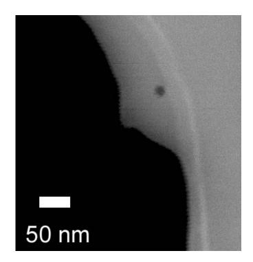
**Figure 5.** Helium ion micrograph imaged with the secondary electrons of a hole etched into a multi layer graphene flake (grey) on a  $SiO_2$  substrate (black).
