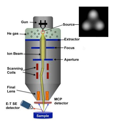
**Figure 1.** Schematic of the Zeiss ORION helium ion microscope column, showing the ion source, apertures, Everhart-Thornley secondary electron (E-T SE) detector and microchannel plate (MCP) detector configuration. (Inset) Image of atomic trimer on a tungsten tip, where ionization occurs.
