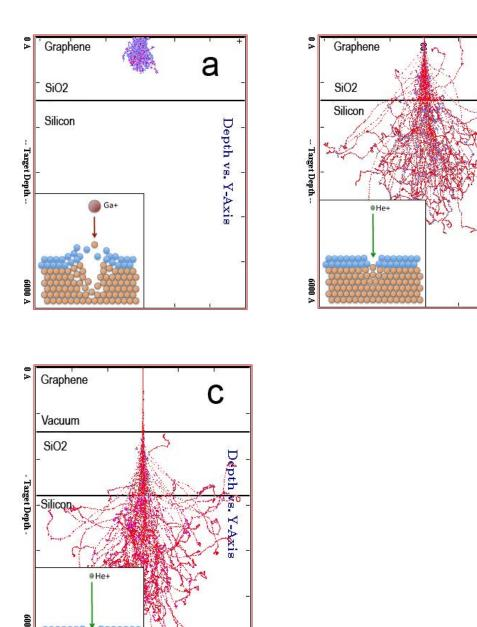
**Figure 3**. Simulations using TRIM software [10] comparing a) 30 kV Ga ions and b) 30kV He ions for range and trajectory in graphene layers on SiO<sub>2</sub> on silicon substrate. c) Range and trajectory of 30 kV He ions through a suspended graphene layer over vacuum, SiO<sub>2</sub> and silicon substrate. (Insets) Schematic comparison between Ga+ ion and He+ ion interaction with graphene samples from molecular dynamics simulations [11].
