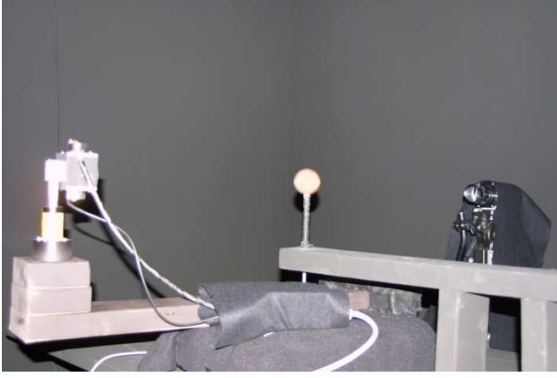
Figure 2: A photograph of our high-speed BRDF measurement gantry.
