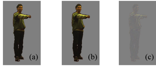
Figure 5: Average coding illustrated with a texture example. a) Masked camera input image; b) Masked reference frame; c) Masked delta frame.
