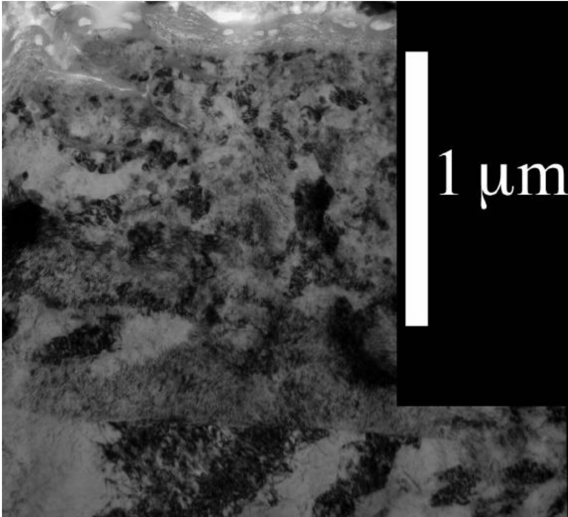
Fig. 7. Cross-sectional transmission electron microscopy image of sample Mo2 that had a 1.4 \mu\text{m} melt depth.
