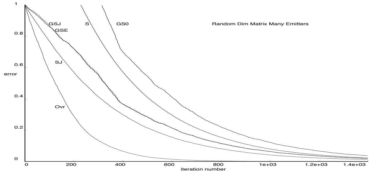
Figure 8: Error at each iteration, random dim matrix with many emmiters
