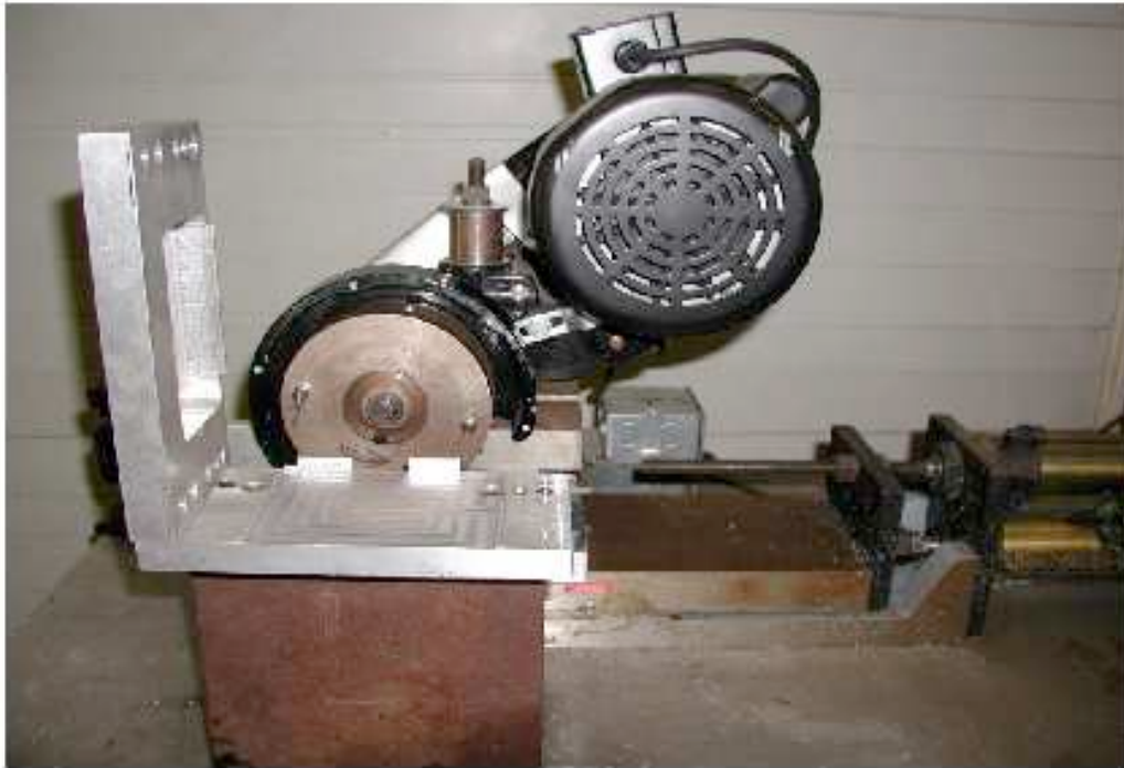
Fig. 16. The fly-cutting machine, shown with its safety shield removed for clarity. The flywheel with diamond bits can be seen behind an L-shaped clamping fixture used to hold the optical connector at a precise location. Smooth transverse motion across the optical face is provided by the pneumatic drive located at the lower right in this photograph.
