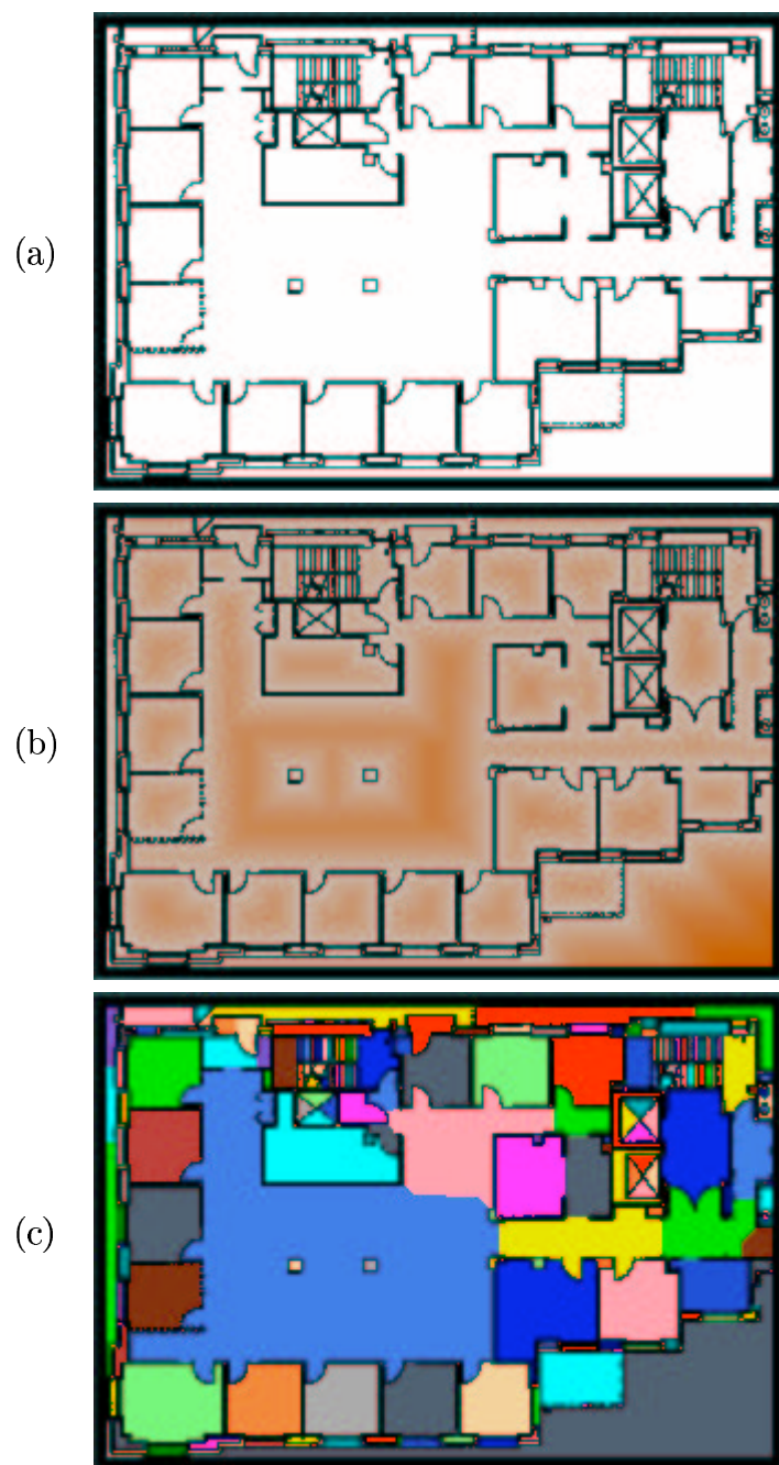
Figure 3: Sample scanned bitmap. (a) The original bitmap. (b) The false-colored proximity field generated for the bitmap. (c) The regions delineated according to the proximity map in (b).
