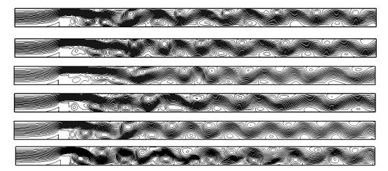
Fig. 11. Example 3.4, streamlines of the velocity at t = 50 for  $\nu = 10^{-3}$  and  $h = \sqrt{2}/32$ : Eul-ninc1, Eul-ninc2, Eul-inc, BDF-inc, RK-inc, and reference finite element solution (top to bottom), 41 equidistant streamlines in [-1, 3].
