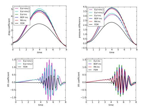
Fig. 15. Example 3.5, computed benchmark coefficients with central differences for discretizing the convective term with  $h = \sqrt{2}/200$ ,  $\Delta t = 10^{-3}$ . The finite element curve is from the reference simulation in [22].
