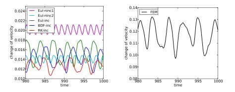
Fig. 8. Example 3.3, change of the Euclidean norm of the computed velocity  $\|\tilde{u}^{n+1} - \tilde{u}^n\|_{l^2}$ .
