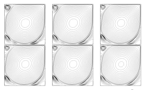
Fig. 9. Example 3.3, streamlines of the velocity for  $\text{Re} = \nu^{-1} = 10000$ ,  $h = \sqrt{2}/320$ : Eul-ninc1, Eul-ninc2, Eul-inc, BDF-inc, RK-inc, reference finite element solution (top left to bottom right), 20 equidistant intervals in [-0.15, -0.01], 6 equidistant intervals in [-0.01, 0], and 40 equidistant intervals in [0, 0.01].
