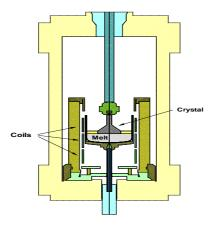
Figure 1: Schematic representation of a vapor pressure growth arrangement of the Institute of Crystal Growth (IKZ) Berlin.
