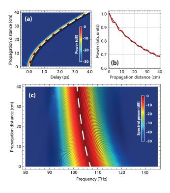
Figure 3: Space-time (a) and spectral (c) representation of a single soliton propagating along the fiber under influence of Raman effect from numerical simulation using full GNLSE. Additional dashed lines result from the adiabatic equations (7–9). (b) Soliton's peak power from the GNLSE (red) and from the adiabatic equations (dashed). See Sec. 3 for parameters.
