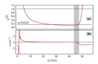
Figure 4: (a) Pairs of  $\Omega$  and relative DW amplitude  $\sqrt{\mu}$  for which solitons frequency does not change. Amplitude is plotted instead of power to facilitate readability. (b) Stability analysis. The region of stable SSFS compensation is shaded gray.
