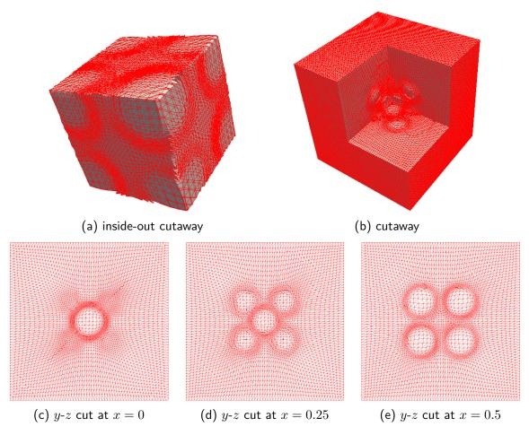
Figure 9: Adaptive mesh example and y-z plane cuts for Example 4.4
