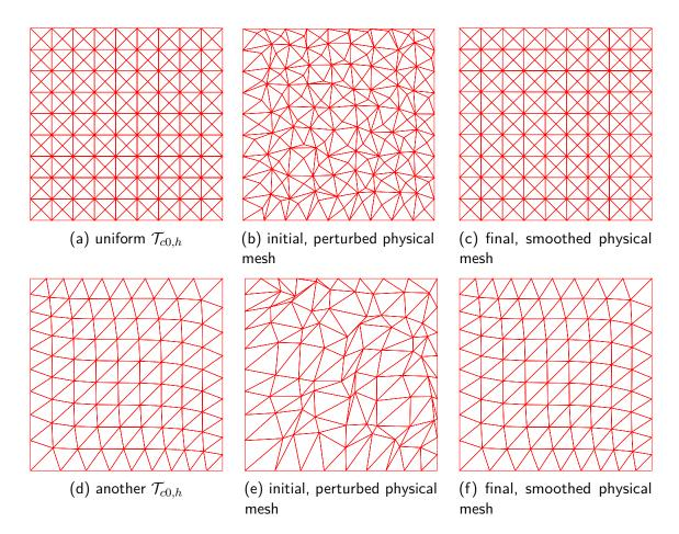
Figure 2: Mesh examples for mesh smoothing in Example 4.1
