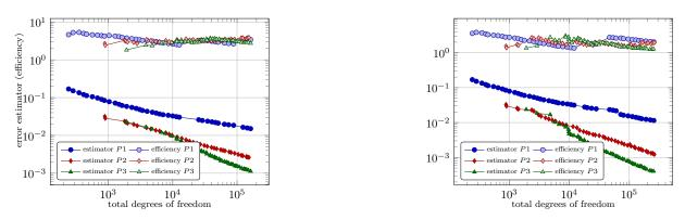
FIGURE 1. Convergence of the error estimator in the energy norm with FEM of degree 1,2 and 3 for the stationary diffusion problem on the square with homogeneous Dirichlet boundary conditions for slow ( $\tilde{\sigma} = 2$ , left) and fast ( $\tilde{\sigma} = 4$ , right) decay. Total number of degrees of freedom and efficiency of the error estimator with respect to the MC reference error.
