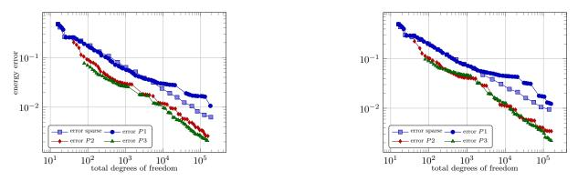
FIGURE 10. Convergence of the error in the energy norm for the stationary diffusion problem on the L-shaped domain with homogeneous Dirichlet boundary conditions for slow ( $\tilde{\sigma} = 2$ , left) and fast ( $\tilde{\sigma} = 4$ , right) decay. Comparison of ASGFEM1 (sparse) and ASGFEM2 for polynomial degrees 1,2 and 3.
