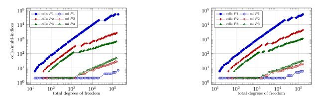
FIGURE 7. Number of mesh cells and active multi-indices with FEM of degree 1,2 and 3 for the stationary diffusion problem on the L-shaped domain with homogeneous Dirichlet boundary conditions for slow ( $\tilde{\sigma} = 2$ , left) and fast ( $\tilde{\sigma} = 4$ , right) decay with respect to total number of degrees of freedom.
