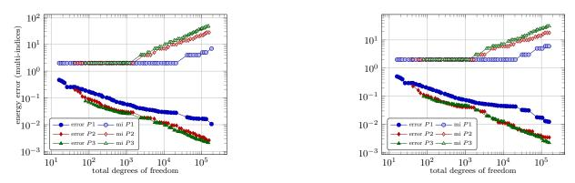
FIGURE 6. Convergence of the error in the energy norm with FEM of degree 1,2 and 3 for the stationary diffusion problem on the L-shaped domain with homogeneous Dirichlet boundary conditions for slow ( $\tilde{\sigma} = 2$ , left) and fast ( $\tilde{\sigma} = 4$ , right) decay. Total number of degrees of freedom and active multi-indices.
