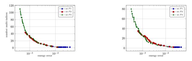
FIGURE 4. Number of active multi-indices with FEM of degree 1,2 and 3 for the stationary diffusion problem on the square domain with homogeneous Dirichlet boundary conditions for slow ( $\tilde{\sigma} = 2$ , left) and fast ( $\tilde{\sigma} = 4$ , right) decay with respect to the energy error.
