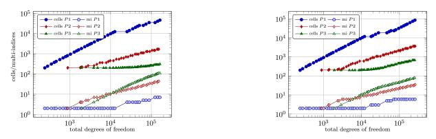
FIGURE 3. Number of mesh cells and active multi-indices with FEM of degree 1,2 and 3 for the stationary diffusion problem on the square with homogeneous Dirichlet boundary conditions for slow ( $\tilde{\sigma} = 2$ , left) and fast ( $\tilde{\sigma} = 4$ , right) decay with respect to total number of degrees of freedom.
