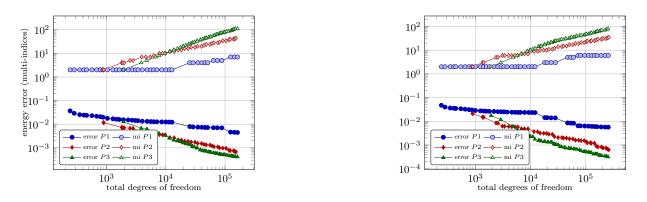
FIGURE 2. Convergence of the error in the energy norm with FEM of degree 1,2 and 3 for the stationary diffusion problem on the square with homogeneous Dirichlet boundary conditions for slow ( $\tilde{\sigma} = 2$ , left) and fast ( $\tilde{\sigma} = 4$ , right) decay. Total number of degrees of freedom and active multi-indices.
