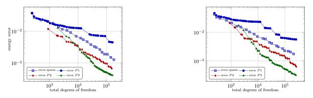
FIGURE 9. Convergence of the error in the energy norm for the stationary diffusion problem on the square domain with homogeneous Dirichlet boundary conditions for slow ( $\tilde{\sigma} = 2$ , left) and fast ( $\tilde{\sigma} = 4$ , right) decay. Comparison of ASGFEM1 (sparse) and ASGFEM2 for polynomial degrees 1,2 and 3.
