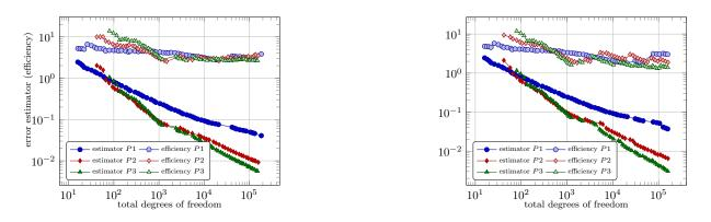
FIGURE 5. Convergence of the error estimator in the energy norm with FEM of degree 1,2 and 3 for the stationary diffusion problem on the L-shaped domain with homogeneous Dirichlet boundary conditions for slow ( $\tilde{\sigma} = 2$ , left) and fast ( $\tilde{\sigma} = 4$ , right) decay. Total number of degrees of freedom and efficiency of the error estimator with respect to the MC reference error.
