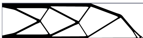
FIGURE 6. A long cantilever beam with low material fraction and a low interfacial energy penalization.
