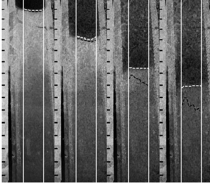
Figure 6: The suspension flow with \phi_0 = 0.3 and \alpha = 25^\circ at different stages; time increases left to right; the black and white dashed lines show the clear liquid and particle front positions; the black tick-marks on the side of the track are 5\text{cm} apart; darker regions in the particulate bed indicate higher particle numbers.
