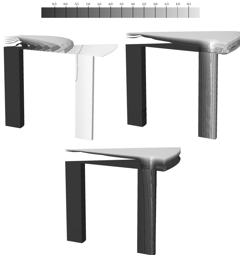
Figure 6: Concentration (in \text{mol/m}^3 ) for flow rates 0.5 \text{ mm}^3/\text{s} (left), 10 \text{ mm}^3/\text{s} (middle) and 80 \text{ mm}^3/\text{s} (right). Isosurfaces ( c = 1.0, 2.0 \dots 6.0 ) are shown in the interior of the working chamber. The anode is situated on the top. Isolines and grayscale color code at surfaces are shown at the inlet (left) and the outlet (right), and the bottom of the working chamber. For the purpose of better visualization, the graphical representation has been stretched by a factor around 10 in z direction compared to the original device.
