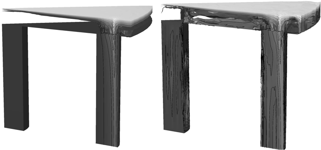
Figure 8: Concentration profile for flow rate 80\text{mm}^3/\text{s} on coarse grid: Scott-Vogelius (top) and Taylor-Hood (bottom). For the explanation of the visualization settings, see Fig. 6.
