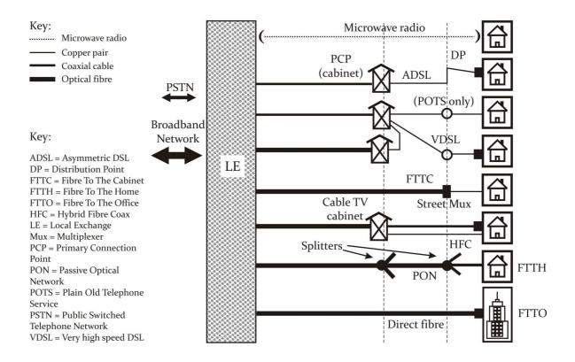
Figure 2.1 - Broadband options for the access network (Source: Valdar, 2006, p. 110)
