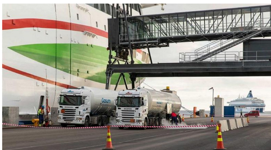
Figure 7. Truck-to-ship bunkering in the Port of Helsinki.
