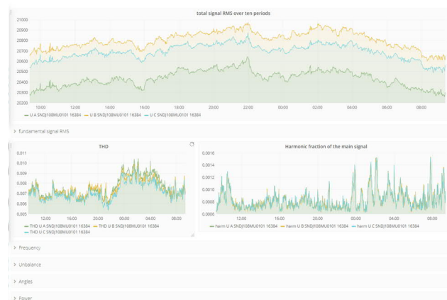
Figure 5. Screenshot of the interface of the DAGR tool displaying power quality parameters.
