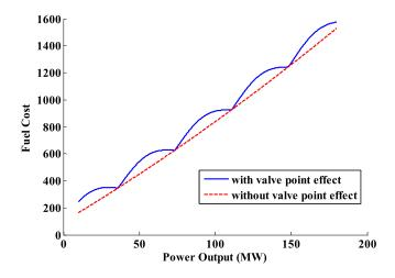
Fig. 1. Cost function with/without the valve point effect.
