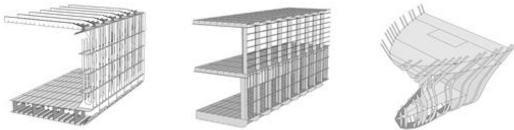
Figure 11. The geometry of the inner structure of: (left) the coastal oil tanker; (middle) the RoPax ship; and (right) the bulbous bow section of the striking tanker ship.
