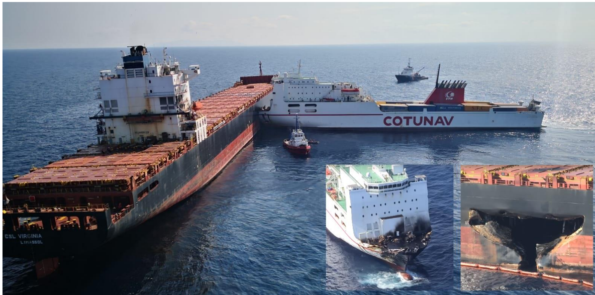
Figure 7. Collision between Ro-Ro Ulysse and containership CSL Virgin Star (Marine Nationale, 2018).
