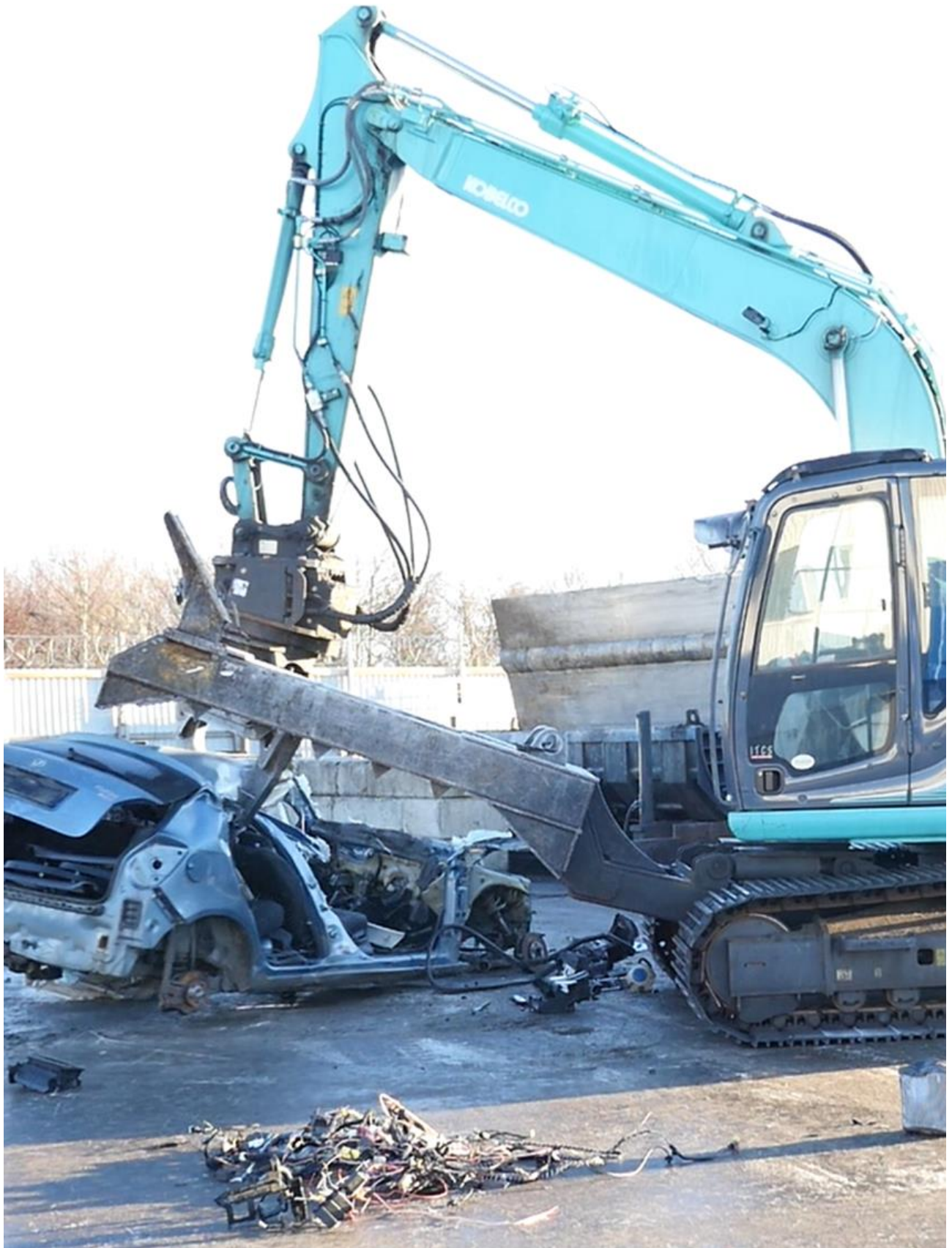
Figure 4: Example of advanced material handling of ELV:s, available only at a few large dismantlers in Sweden today.
