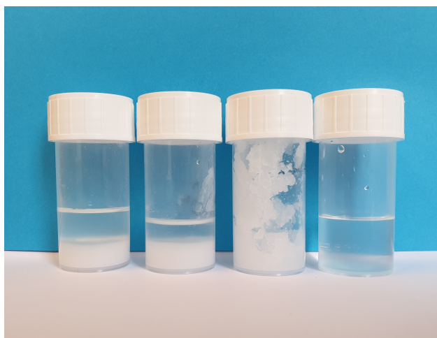
Figure 5.1: From left to right: 3 wt.% MCC in 4 mol%(aq) solution of 50/50 KOH/TMAH, 50/50 KOH/NaOH, 50/50 NaOH/TBAH and 50/50 NaOH/TMAH
