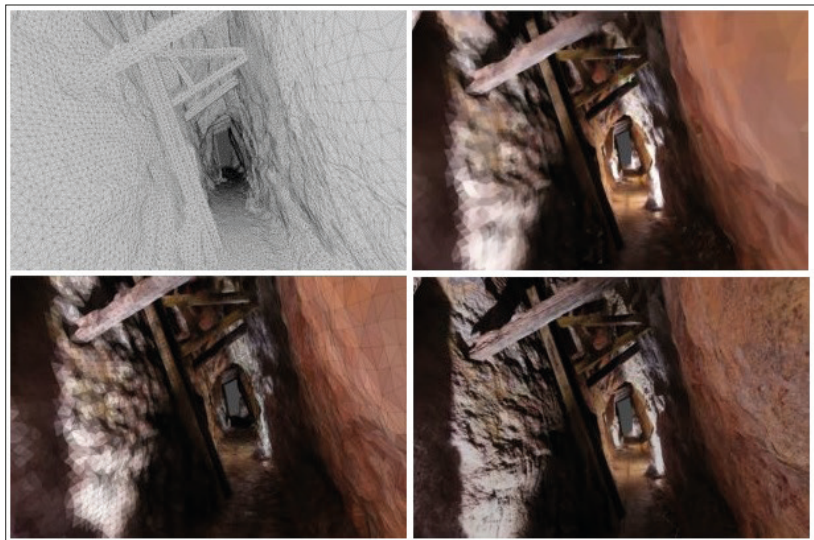
Figure 3. Stages of rendering a 3D model of a tin mine tunnel. Source: EESAB.
