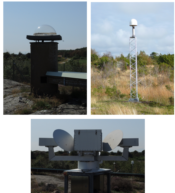
Figure 1: The GNSS installations ONSA (top, left) and ONS1 (top, right) and the WVR Konrad (bottom).
