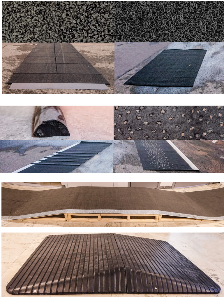
Figure 2. The haptic nudges used in the test. From top and left to right, Soft surface, Spongy Surface, Soft Stripes, Rugged surface, Slope and Soft bump.
