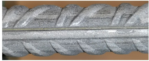
Figure 2. Close up view of the optic fiber sensor attached to a steel reinforcing bar used in the experimental tests.
