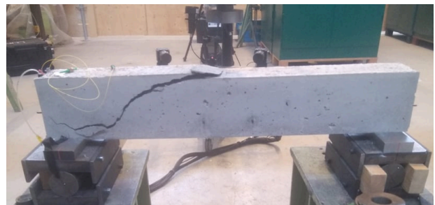
Figure 3. Tested beam after failure.
