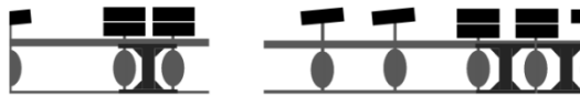
Fig. 3. Different type of trucks with three axis (six wheels) and five axis (ten wheels).
