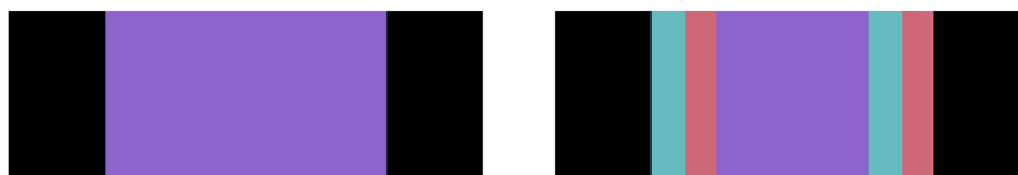
Fig. 2. A simplified schematic of a supercapacitor. In both figures, the electrodes are black and the bulk electrolyte is purple. On the left is the supercapacitor in a state of discharge. On the right hand side, the bulk electrolyte (purple) has formed a double layer of anions (red) and cations (blue) on the surface of the electrodes. (For interpretation of the references to color in this figure legend, the reader is referred to the Web version of this article.)
