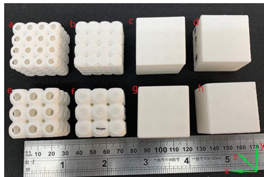
Fig. 3. Fabrication using the material extrusion process: figures (a) and (e) is SU inspired open cell lattice structure with different lattice size, figures (b) and (f) is SU inspired local closed cell lattice structure with different lattice size, figures (c) and (g) SU inspired global closed cell lattice structure with different lattice size, figures (d) and (h) is honeycomb global closed cell lattice structure with different lattice size. The Z-direction arrow represents the build direction.
