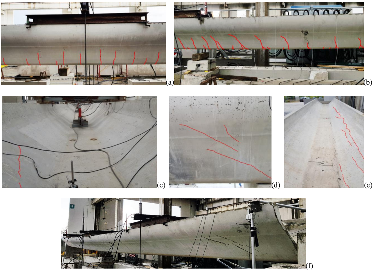
Figure 7 – Evolution of the experimental crack pattern: (a) vertical flexural cracks at midspan; (b) inclined flexural-shear cracks between midspan and the support; (c) crack near the support at element extrados; (d) inclined shear cracks at the support; (e) longitudinal cracks at mid-height of wing extrados; (f) loss of shape of the open cross section in its own plane.
