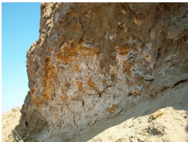
Fig. 4 Sulphate minerals on the slope of the tailing pile
