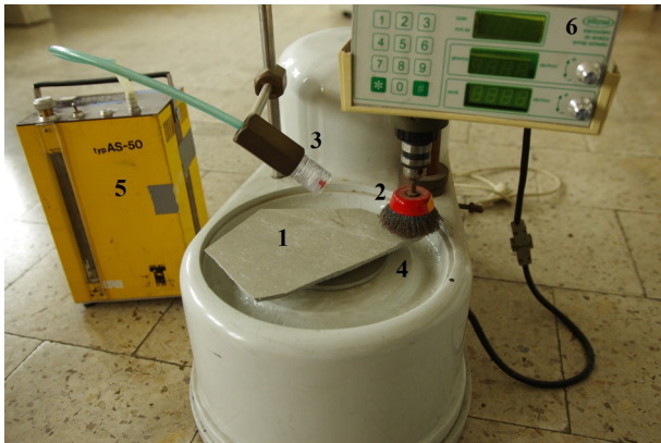
Fig. 2. The experimental set up. (1) AC sheet. (2) Steel wire brush. (3) Filter cassette. (4) Rotating sample holder. (5) Air pump. (6) Electronic controller used to synchronize the frequency of rotation of sample holder and wire brush.
