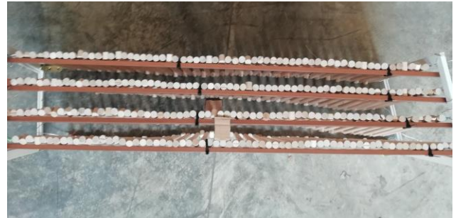
Figure 6 - Aerial view of the metamaterial barrier.
