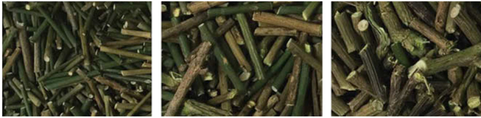
Fig. 2. Detail of the pieces of broom branches after drying, grouped by diameter. On the left with a diameter of 1.5 mm, in the center with a diameter of 3 mm, on the right with a diameter of 4 mm.
