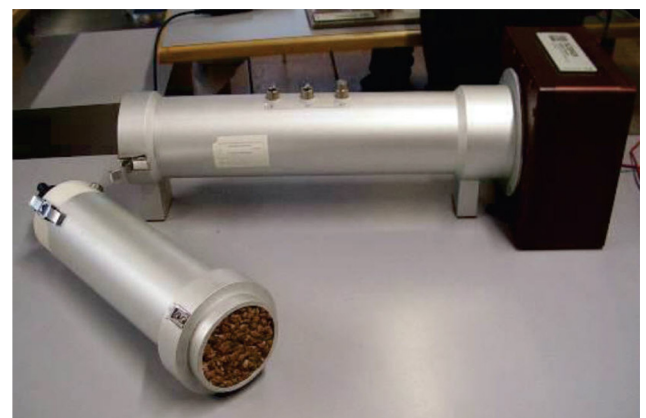
Fig. 4. Tube of Kundt, for the absorption coefficient measurements.
