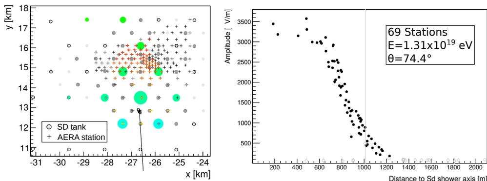
**Figure 5.** Example event of a horizontal air shower with the current AERA set-up. The grid of the surface detector stations and antenna stations can be seen on the left and on the right the radio lateral distribution can be seen. The color scheme of the SD tanks and the AERA stations on the left indicate the timing information of the triggered tanks and stations and thus the arrival direction of the shower. The size of the circles indicates the signal strength.
