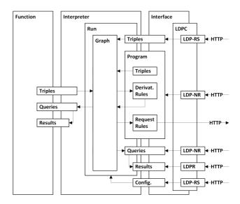
Figure 3.6: Smart Component - Architecture
