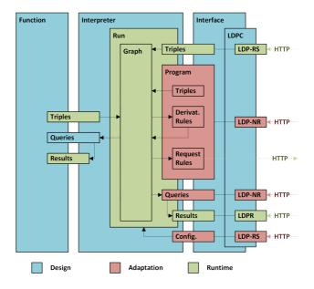
Figure 3.9: Smart Component - Architecture: Separation of Lifecycles
